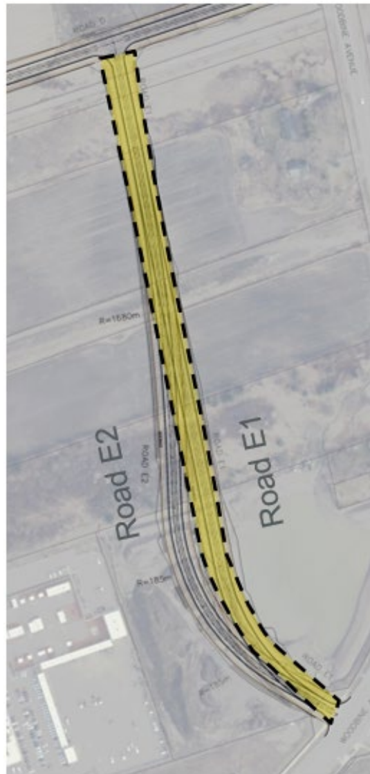
Exhibit 5-9: Preliminary Recommended Collector Road E1 Alignment
