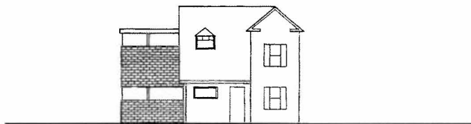
Incompatible contrast: addition is too contrasting; draws attention; compromises integrity of existing building.
