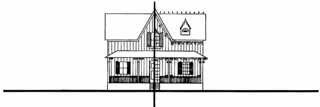
A heritage building with original, simple architectural details compared to the introduction of new elaborate architectural details uncommon to Unionville.
