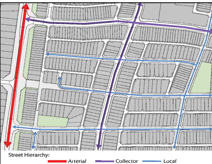
Coordination of traffic hierarchy with public amenity on the main street (top); Diagram of street hierarchy (bottom).
