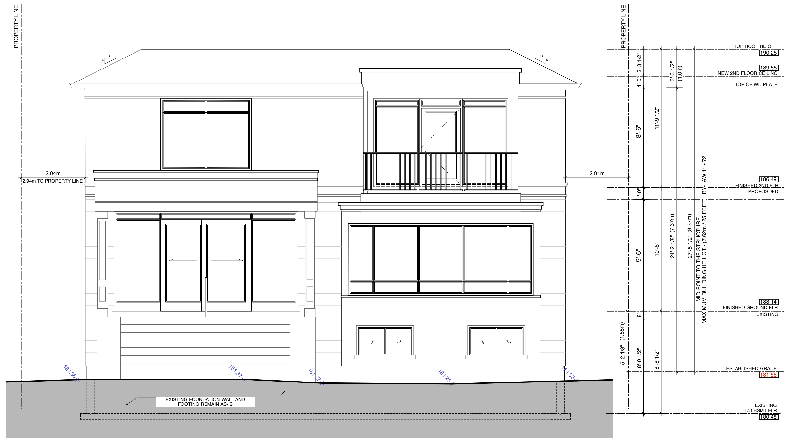
1 SOUTH (REAR YARD) ELEVATION SCALE: 1/4" = 1'-0" ELEVATION LABEL IS BASED ON THE CARDINAL ORIENTATION (CONSTRUCTION NORTH)
