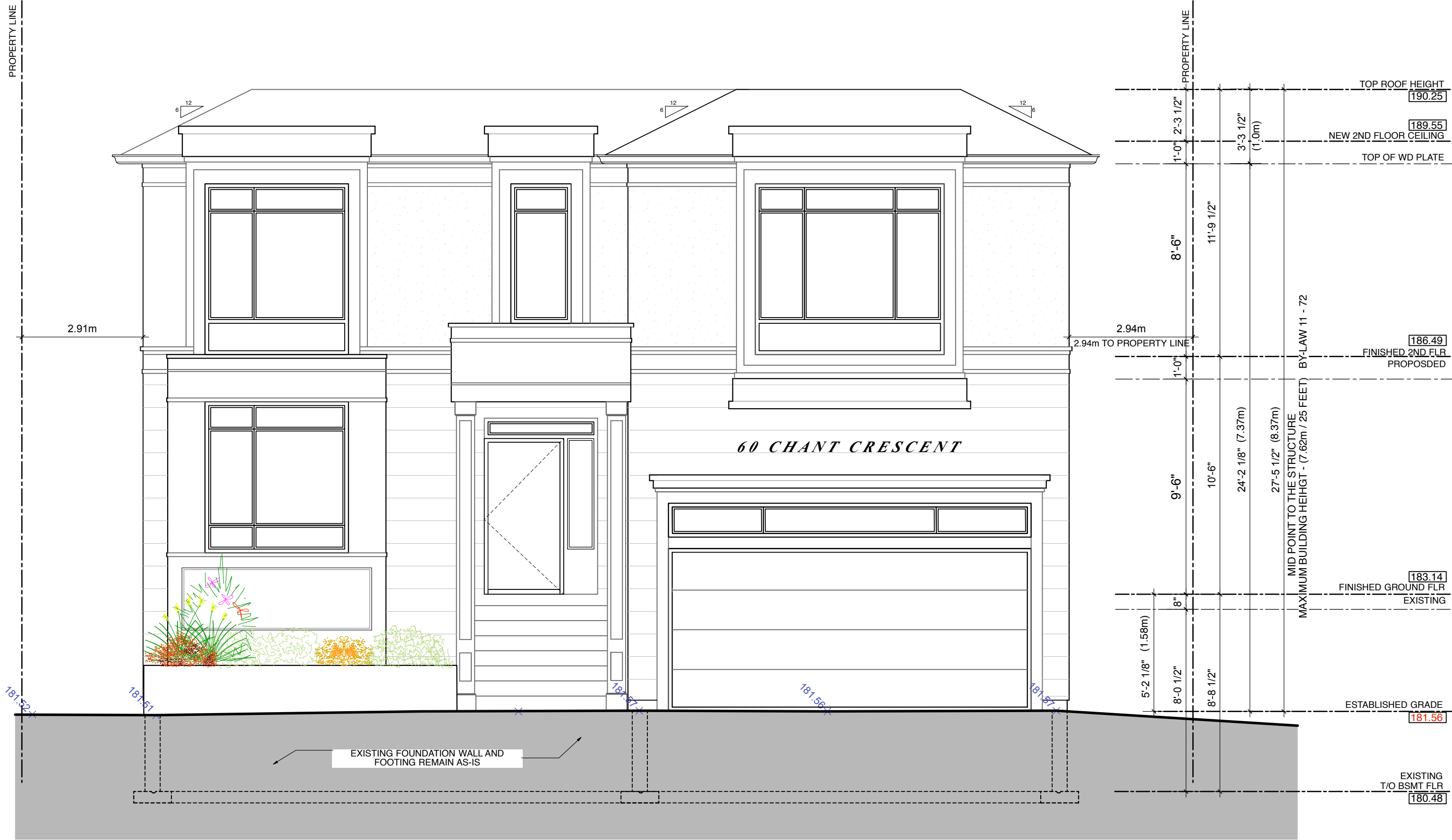
1 NORTH (FRONT YARD) ELEVATION SCALE: 1/4" = 1' - 0" ELEVATION LABEL IS BASED ON THE CARDINAL ORIENTATION (CONSTRUCTION NORTH)
