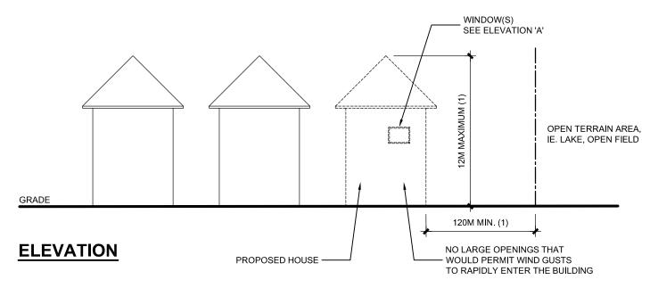
(1) GLASS MUST BE DESIGNED IN CONFORMANCE WITH TABLE 9.6.1.3.D WHEN GREATER THAN 12m MAXIMUM HEIGHT OR LESS THAN 120M MINIMUM.
