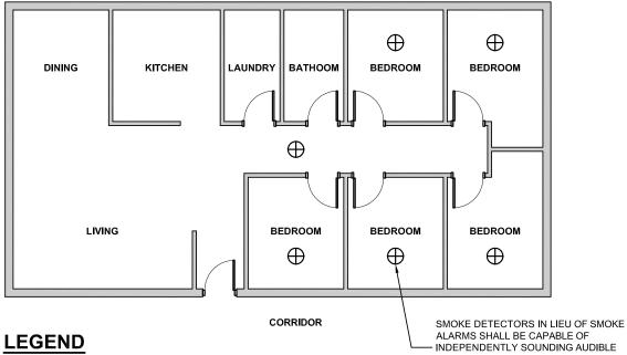
ALARMS SHALL BE CAPABLE OF INDEPENDENTLY SOUNDING AUDIBLE SIGNALS WITHIN THE INDIVIDUAL SUITES CONNECTED TO FIRE ALARM SYSTEM
