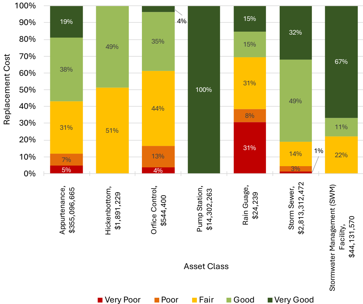
Figure B - 8: Performance Distribution of Stormwater Assets by Asset Class
