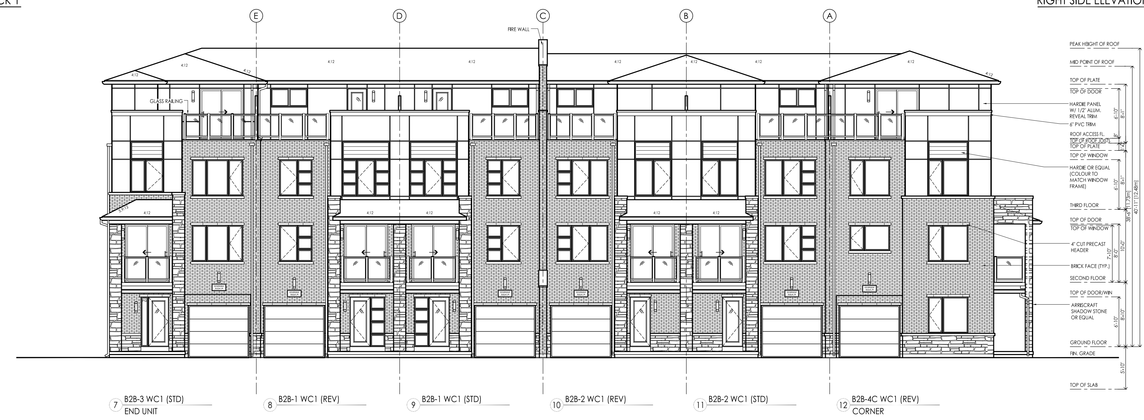
REAR ELEVATION - TYPICAL BLOCK 1 WEST COAST CONTEMPORARY
