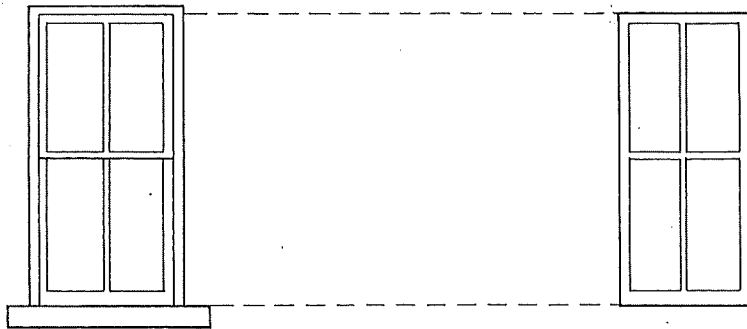
Appropriate: 2/2 storm window added externally to 2/2 original window
