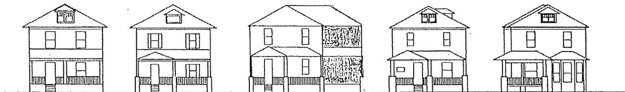
3. Appropriate: The dwelling's scale is reduced through articulation of the façade with part of the dwelling set back. Rhythm, spacing and alignment are based on the existing context.
