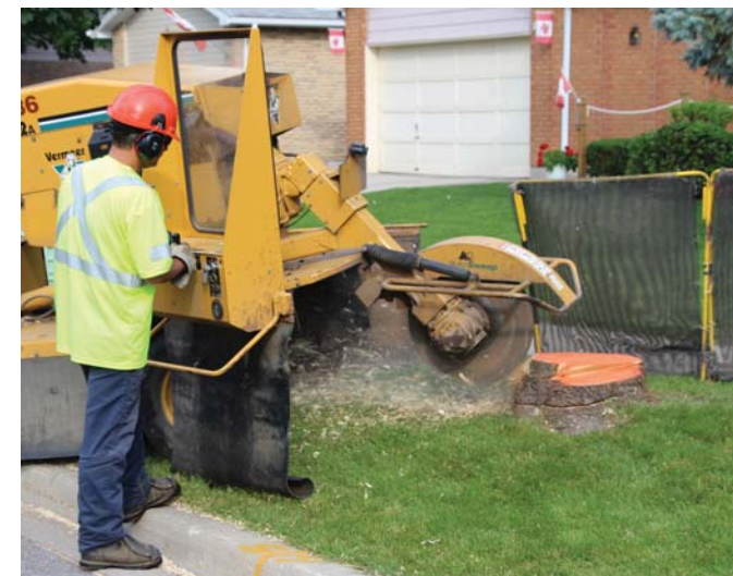
Crews grind tree stumps away (called stumping) in order to replant new trees in the same location, as part of Markham's Emerald Ash Borer Management Plan.
