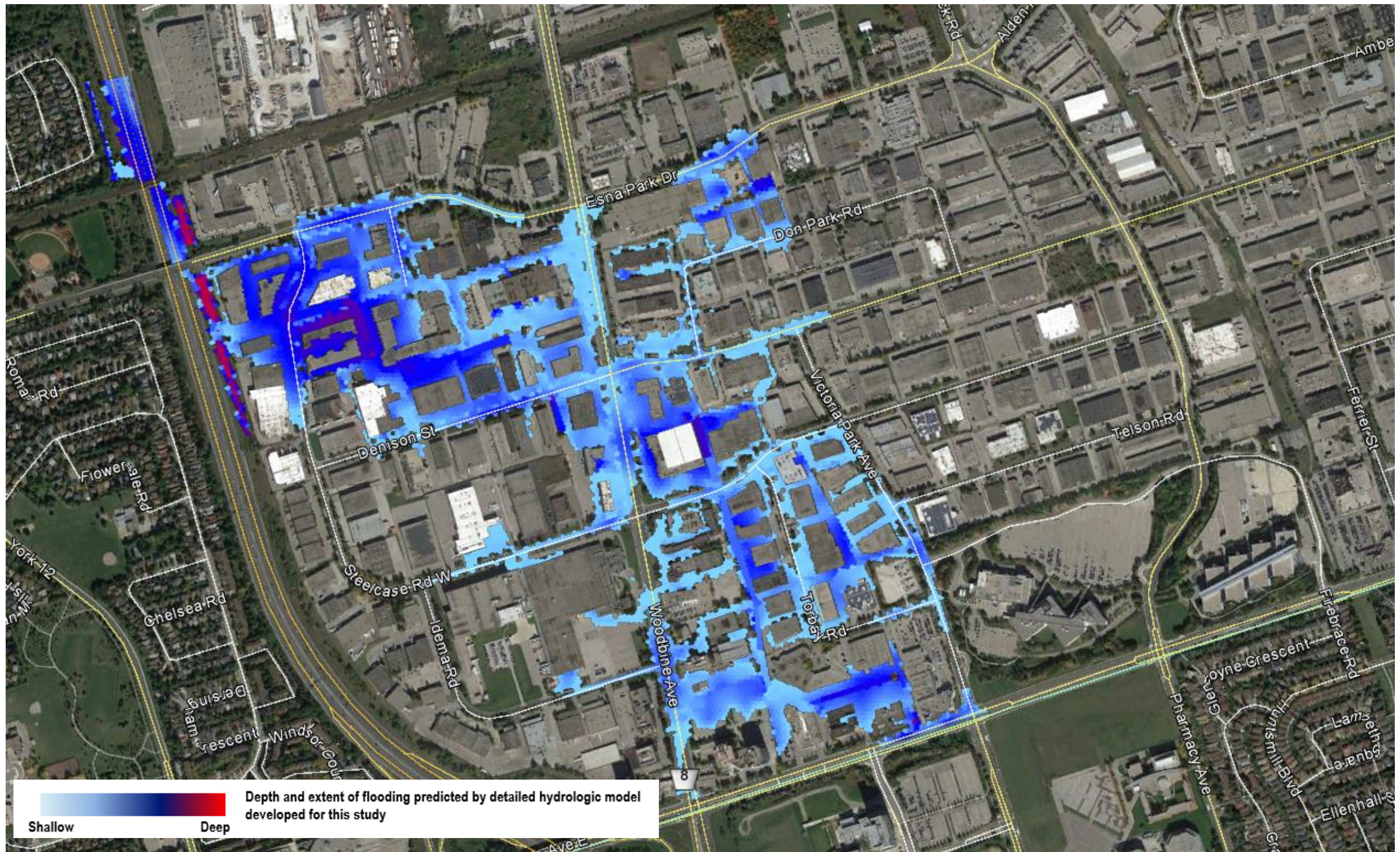
Figure 2-19 Predicted Extent of Flooding – August 19, 2005 Storm
