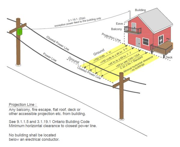
Please note these minimum above clearances includes an additional 1.8m wire swing if the swing is not known. Please check with the P.U.C. concerning voltage of wire and what swing would apply.
