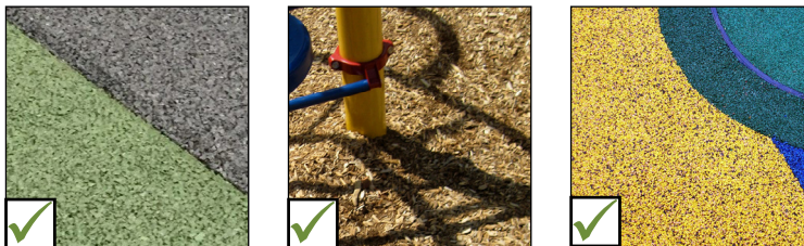
Examples of inclusive play space ground surfaces. From left to right: rubber tile, engineered wood fiber and shredded rubber.
