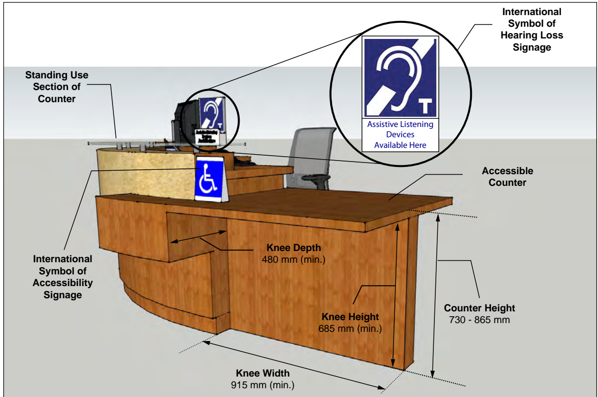
Figure 97b: Accessible Service Counter with Knee Clearances
