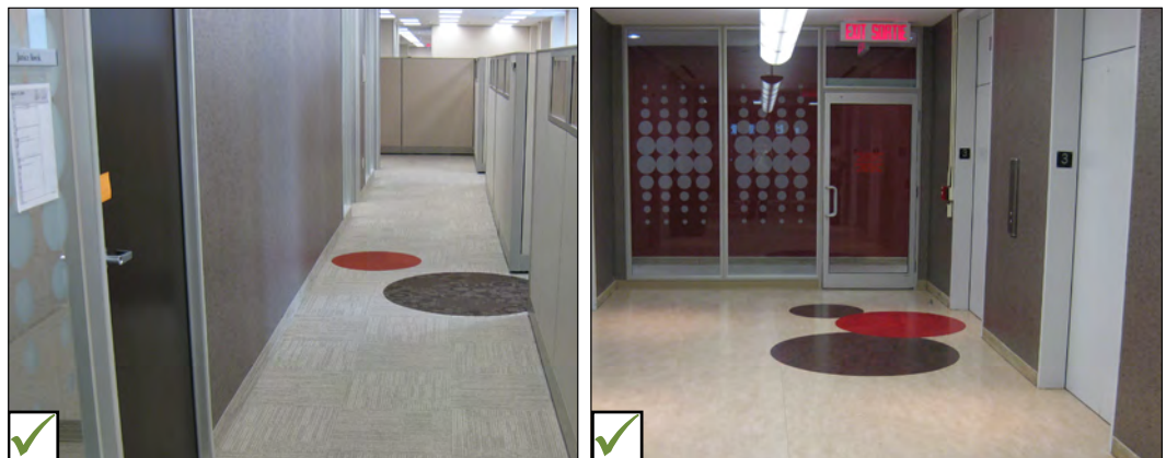
Examples of floor surface and elevator door finishes that minimize glare.
