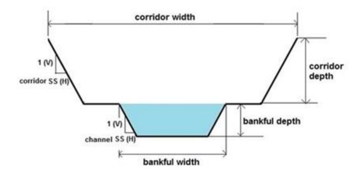
Figure 5. Schematic of representative cross-section.
