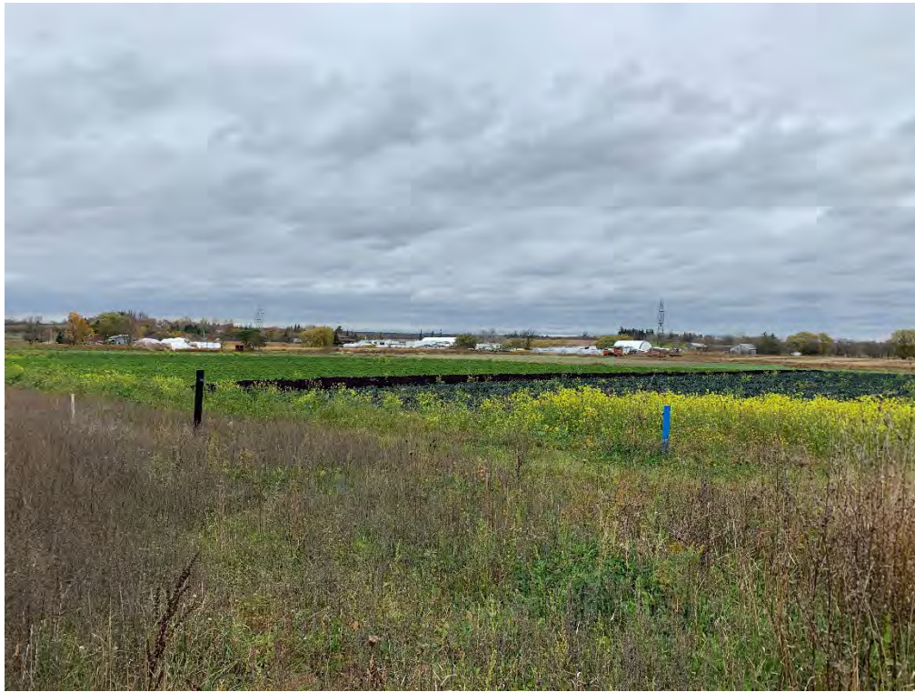
Photo 19: Two monitoring wells located at the southwest corner of the agricultural field located westerly adjacent to 2825 19th Avenue. The monitoring well with black protective casing was installed by Thurber on July 11, 2019.
