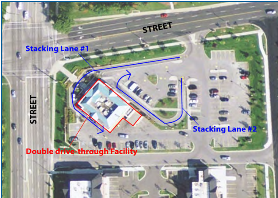
Figure 4.3b: This example illustrates the urban design challenges associated with a double drive-through facility resulting from two stacking lanes addressing one building.
