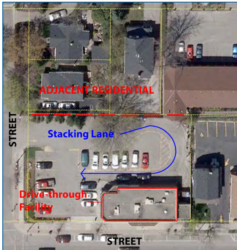
Figure 4.4b: Illustrates inadequate buffering / separation from adjacent residential. The red bold hatched line indicates the commercial and residential interface.
